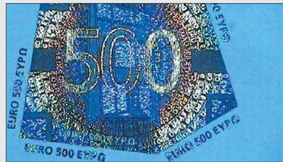
Below: OVDs revealed with LED illumination.
